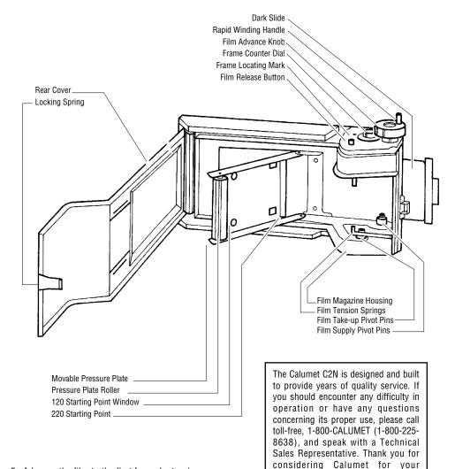
5. Advance the film to the first frame by turning the rapid winding handle until it stops. Insert the C2N holder into the back of the camera, as you would a sheet film holder. Check to make sure your lens' shutter is closed before removing the C2N's dark slide.
