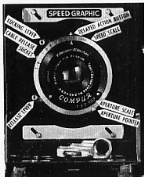
Figure 2c. The Rim-Set Compur Shutter.
